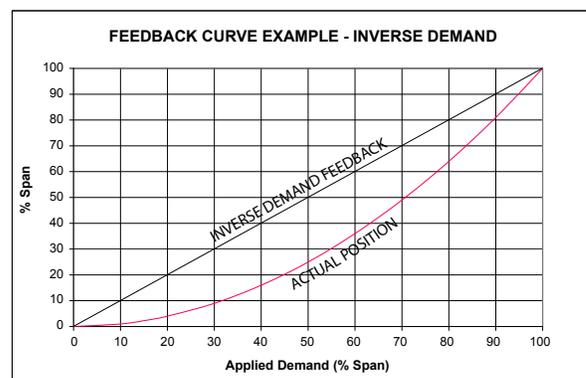
The following methods describe how to enable or disable position Feedback, set the 0% and 100% milliamp values and select the desired Feedback response.
