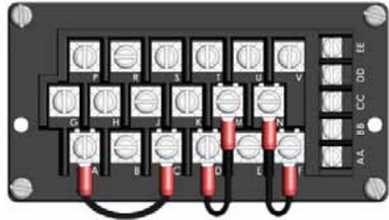
To prevent Handswitch initiated motion, remove jumper (JA) from between terminals A and C.
