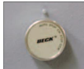
The Demand signal can position the actuator only when the Handswitch is in the AUTO position.
