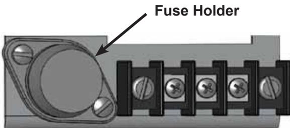
Turn the fuse holder CCW while pressing down. The fuse holder should spring loose when free. Remove the fuse holder from the actuator. Pull the fuse free from the holder. Replace the fuse with the same type (see table below) by pushing it into place.
