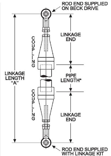
\*NOTE: To calculate length of pipe required, subtract "Length of 2 Linkage Ends" (shown in table above) from Linkage Length "A" (shown in diagram above).
