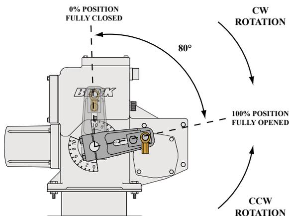
**NOTE:** The crank arm in the figure above may be adjusted to any start angle. The orientation and rotation shown here has been randomly selected for the purpose of this example.
