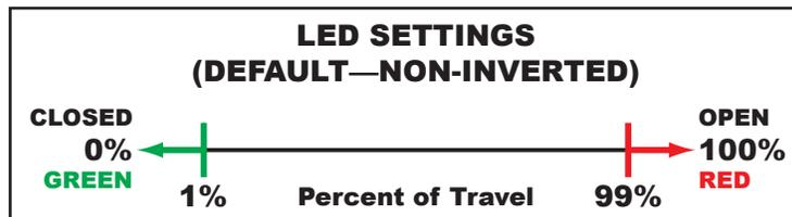
*Example 1: Make the "CLOSED" green LED light at 2.0% and the "OPEN" red LED light at 98.0%.*
