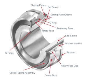
The slurry seal for WEMCO® Torque-Flow® pumps replace standard packing and requires no external flush system. The slurry seal operates in the product being pumped without diluting the product.
