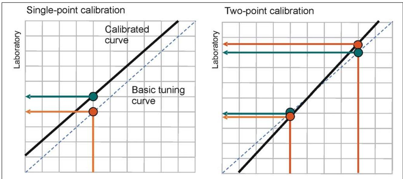
Fig. 2. Single-point and two-point calibration.
