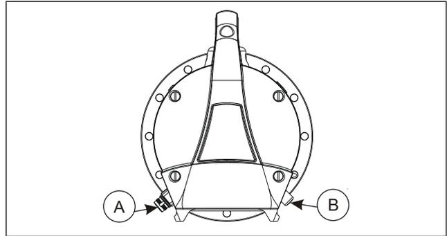
Fig. 3. Metso rotating consistency transmitter, rear view: A. motor cable connector, B. TCU cable connector
