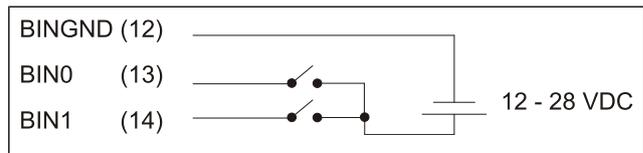
Fig. 9. Connection principle of binary inputs.
