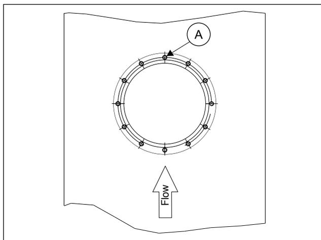
Fig. 8. A. mount the pin bolt here, secure with Loctite.
