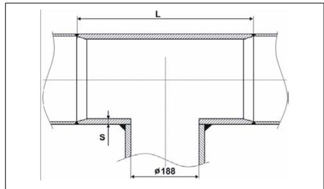
Fig. 2. Pipe replacement section for process pipe sizes DN200...DN800 (see Tables 4, 7).
