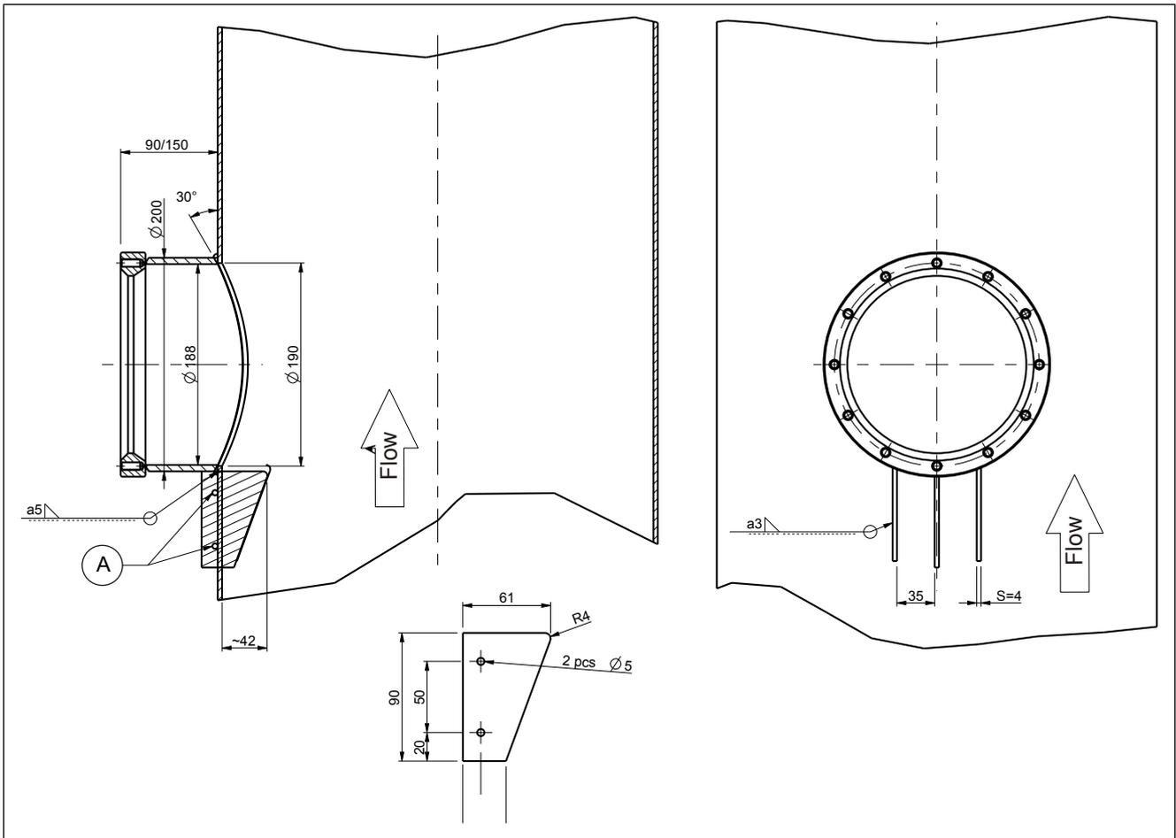
Fig. 9. Installing deflector plates: A. alignment holes.
