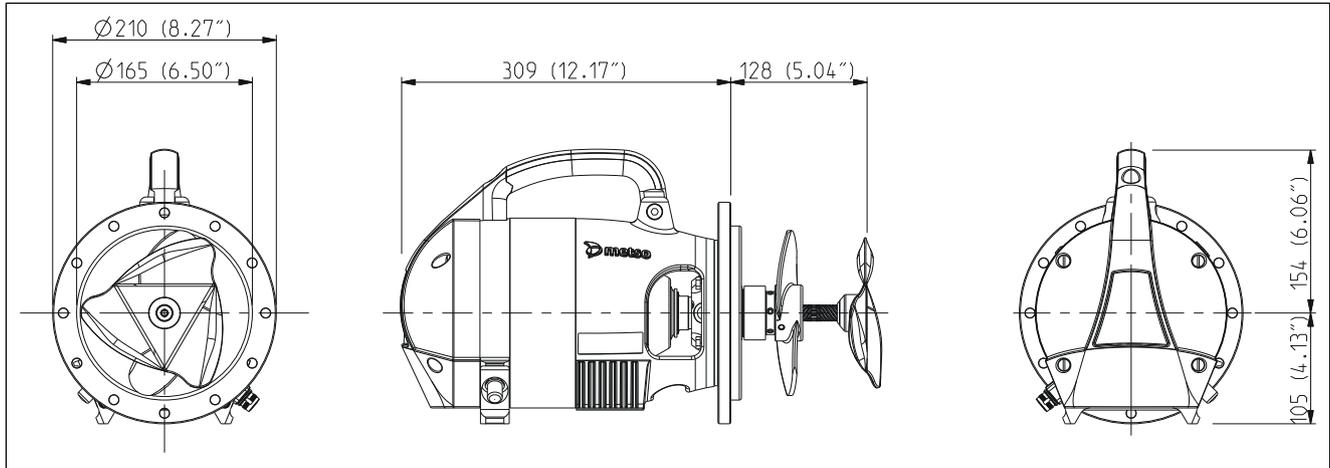
Fig. 3. The dimensions of the transmitter with TH sensing element and small flange, MD model.
