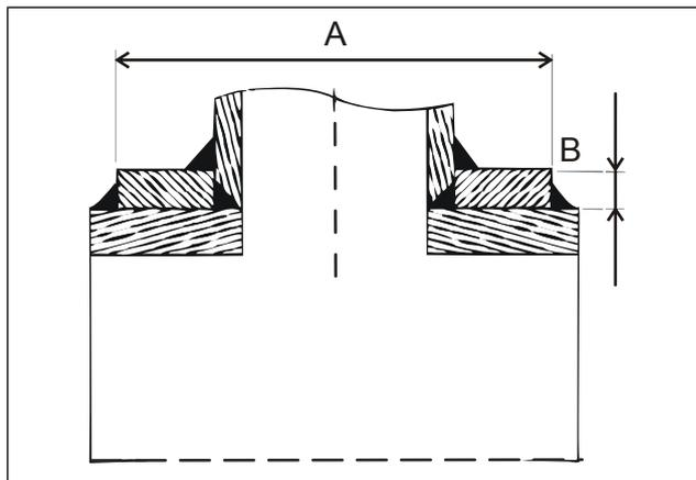
Fig. 3. Reinforcing pad for process pipe sizes DN400...DN800 (see Table 9).
