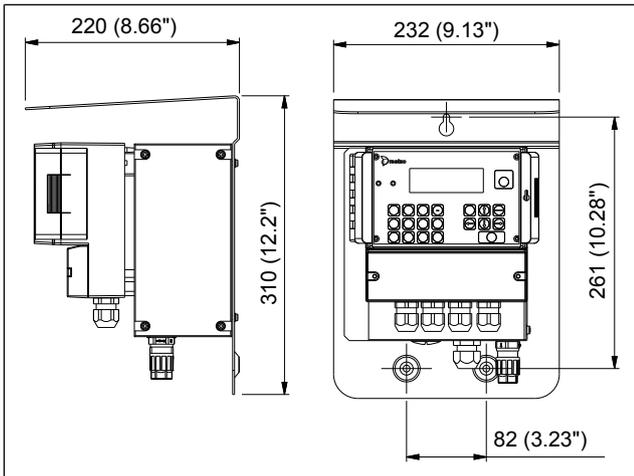
Fig. 2. Mounting dimensions of TCU, MD model of the transmitter (K09176).
