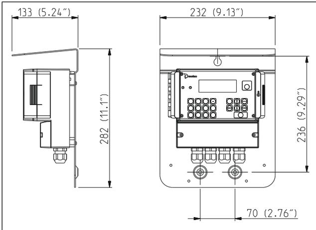
Fig. 1. Mounting dimensions of TCU, BD model of the transmitter (K09173).
