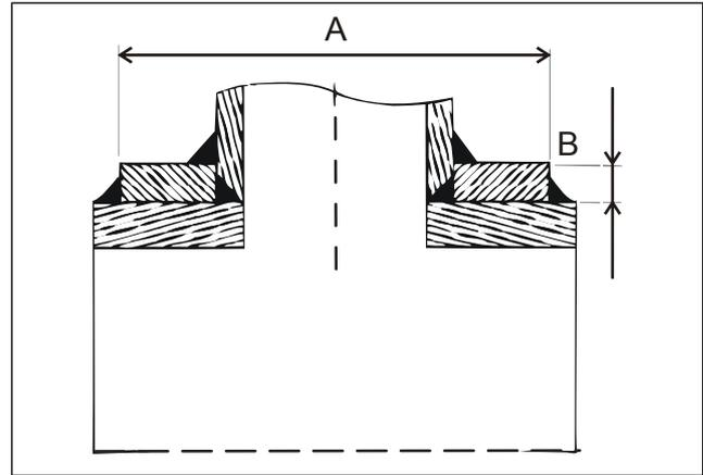
Fig. 1. Reinforcing pad for process pipe sizes DN400...DN800 (see Tables 3, 6).
