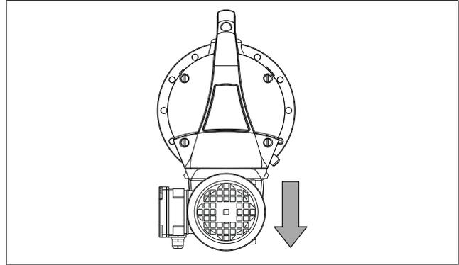
Fig. 12. Motor pointing downwards.
