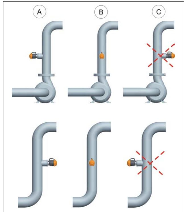
Fig. 4. Transmitter positions.
