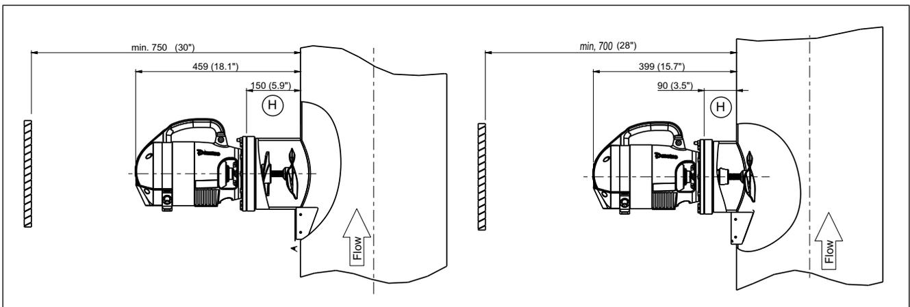
Fig. 10. Profile dimensions of process coupling, H. coupling dimension.
