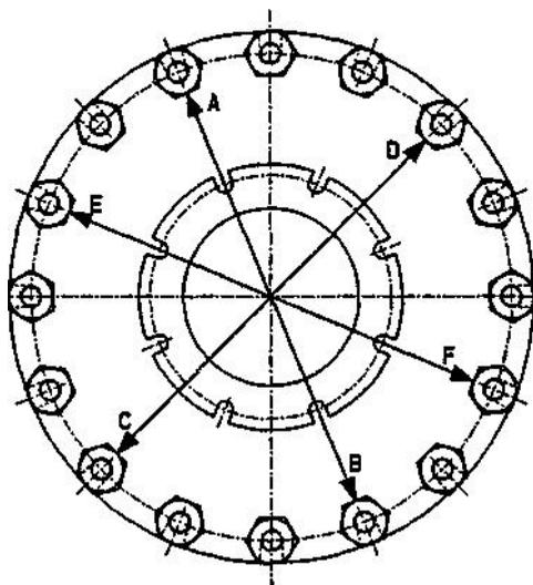
Figure 17: Tighten bolts
