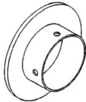
**Figure 16: Bearing holder to install the shaft and bearing assembly into the housing for B3 and B4 frames only**
