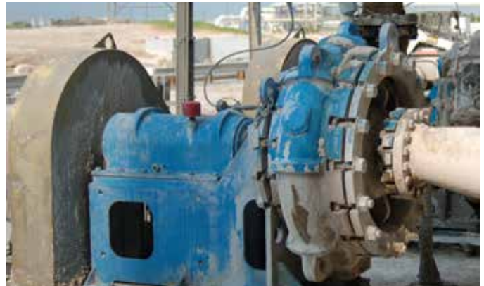
Model 5500 pumping Phosphogypsum in a phosphate plant.
